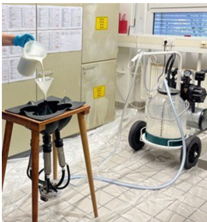
Figure 1: Bucket milking system with milking cluster connected to the rubber udder. Figure 2: Simulations of milkings.
